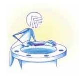
Examine the flange surfaces, fasteners (bolts or studs), nuts and washers to ensure they do not have any serious defects. Replace any components if found to be defective. If in doubt, seek advice.
