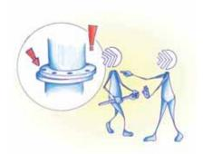
Assure the gasket is the specified size and material and ensure that it is free of defects. Carefully insert the gasket between the dry flanges. Make sure the gasket is centered between the flanges. Do not use joint compounds or release agents on the gasket or seating surfaces unless specified by the gasket manufacturer as this can lead to reduced surface friction.
