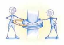
Bring the flanges together ensuring the gasket is not pinched or damaged.
